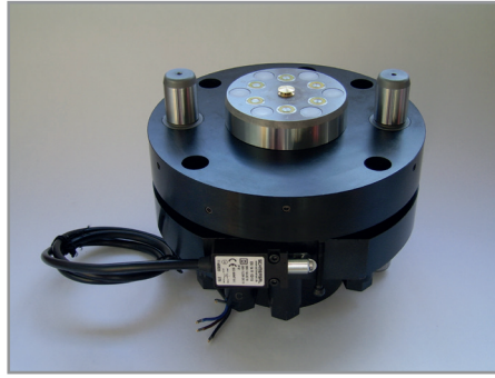
Docking station with six coupling points, pressurized coupling; in order to dock the coupling plate, it is raised by an integrated hydraulic cylinder.
