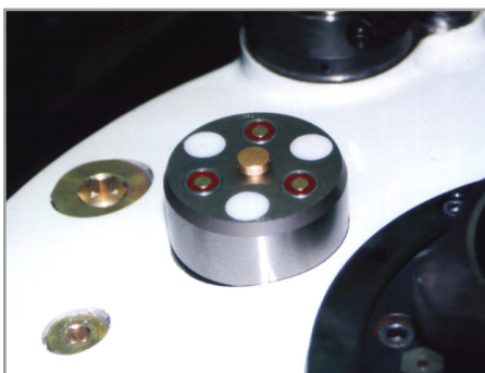
Triple coupling system for hydraulic oil fed of the fixture plate in a machine tool. The connection in the loading and unloading station is realized through the lowering of the fixture plate.
