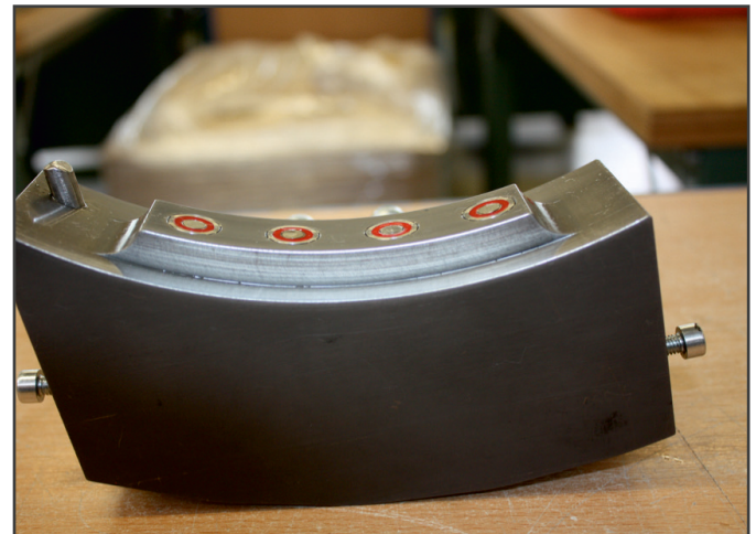
Fixture block with automatic coupling mechanisms
